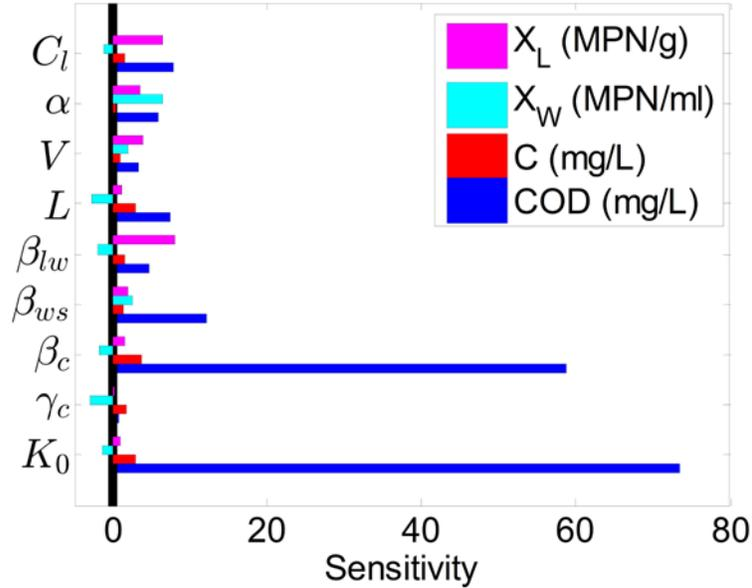
Fig. 11. Sensitivities of the four state estimation errors relative to modeling errors in the nine system parameters
