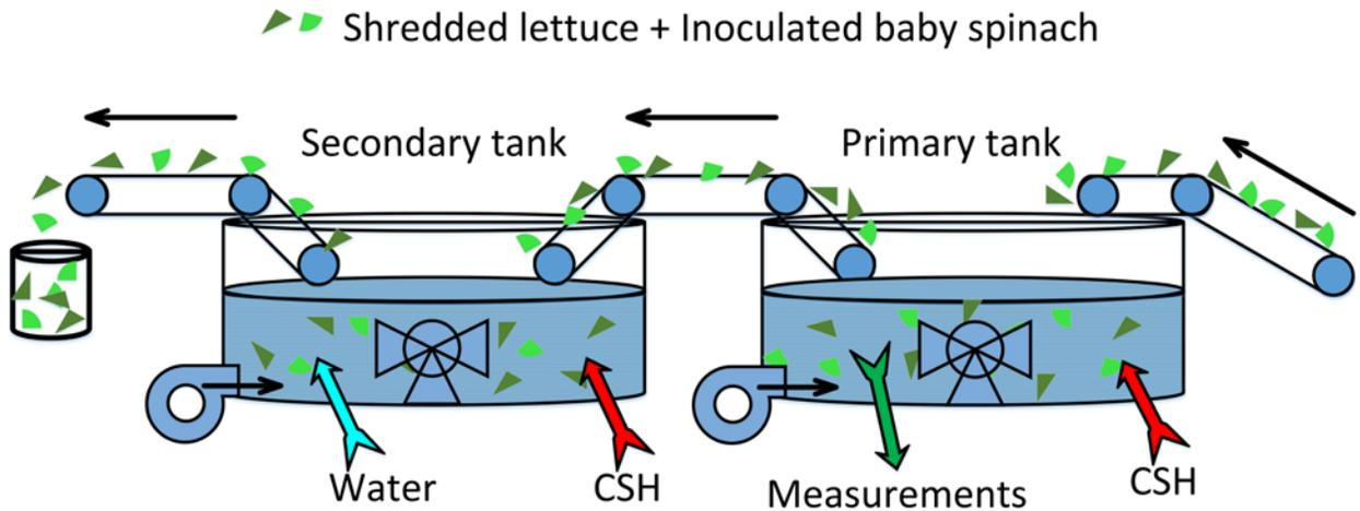
Fig. 1. Commercial double wash system
