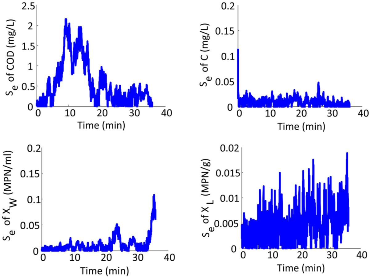
Fig. 10. Standard deviation of the estimation errors for the system states, averaged over 100 Monte Carlo simulations, each with a 36 min simulation time
