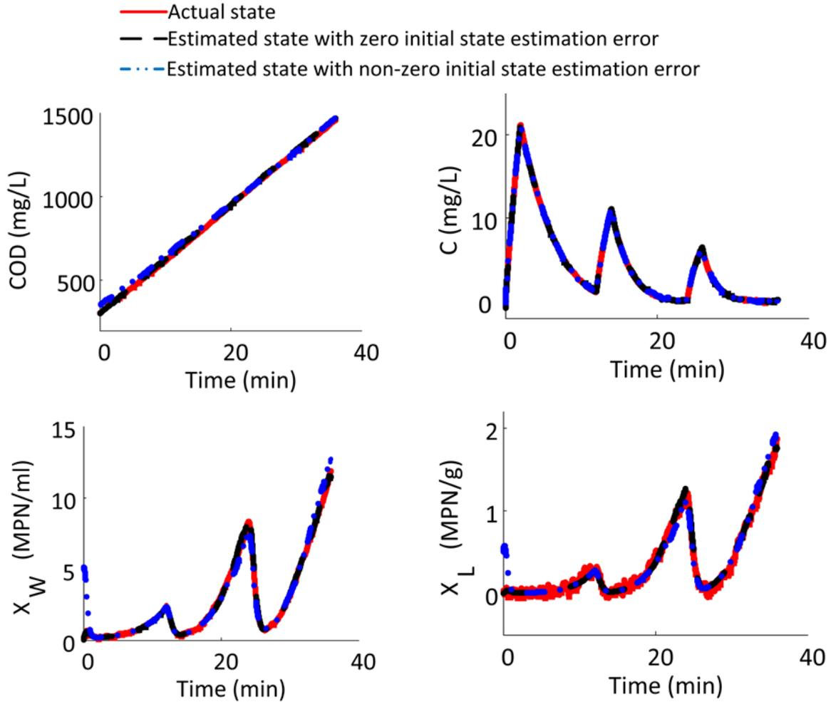
Fig. 6. State estimation performance: simulated states (red solid line), estimated states with zero initial estimation error (black dashed line), and estimated states with non-zero initial estimation error (blue dotted-dashed line)
