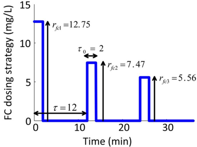
Fig. 2. FC dosing strategy. The magnitude of the FC doses  $r_{fc_i}$ ,  $i = 1, 2, 3$  are calculated in [5] with a least-squares fit to the model of Eq. (1). The dosing width  $\tau_0$  and the FC dosing period  $\tau$  are from [2].
